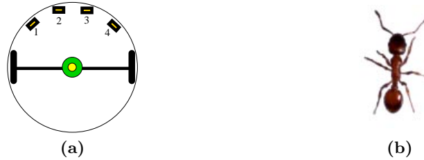
Fig. 2. (a) Sketch of the ant-bot. The circle represents the body. The two elongated rectangles placed on the left and right part of the body denote the wheels of the robot. The four small rectangles on the upper part of the figure shows the placement of the infrared proximity sensors. The concentric circles drawn at the center of the robot indicate the pheromone nozzle and detector. (b) Leptothorax albipennis .
